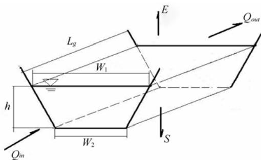
**Fig. 2** Depiction of irrigation canal water balance ( $Q_{in}$  and  $Q_{out}$  are the inflow and outflow rate respectively;  $E$  is evaporation;  $S$  is seepage;  $L_g$  is the length of the segment;  $W_1$  and  $W_2$  are the water surface width and canal bed width, respectively;  $h$  is the water depth.
